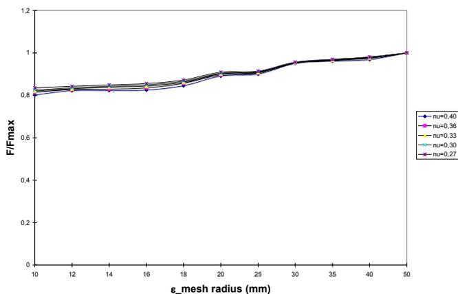
full order 3D mesh ( $F/F_{max}$ ) for different values of the poisson ratio.
