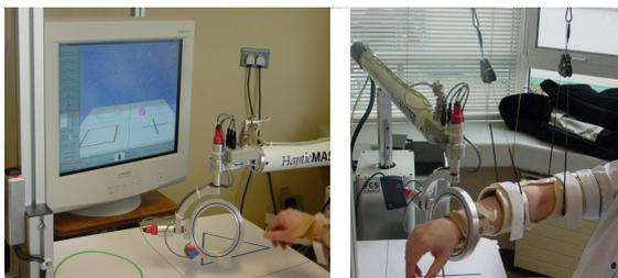
**Figure 2 – Robot end-effector and arm orthosis**
