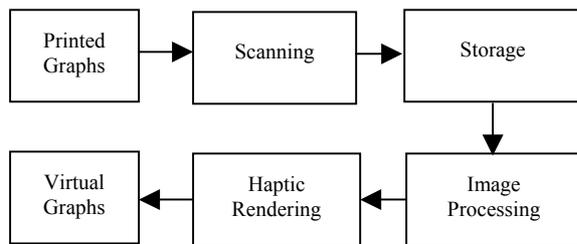
Figure 2. Visual to haptic data conversion process.
