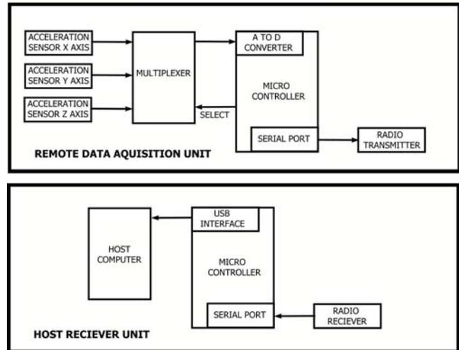
Figure 1. Structure of Prototype System.
