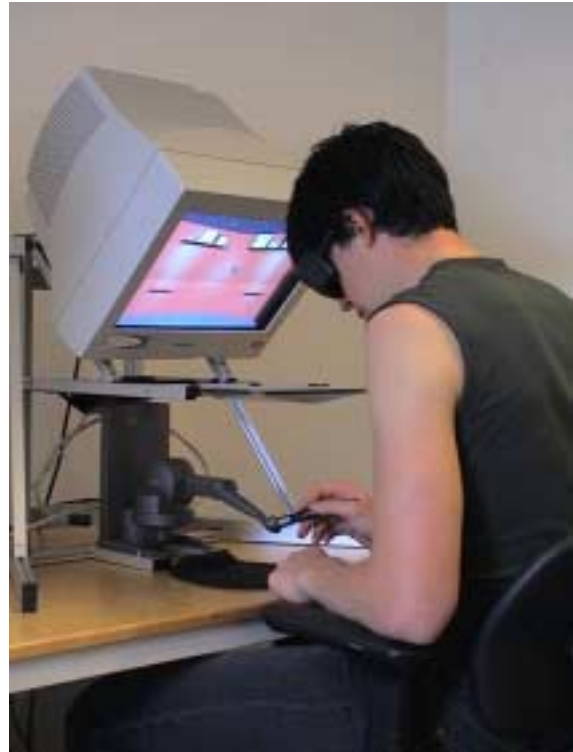
Figure 1. A person collaborating in the haptic collaborative virtual environment using the ReachIn Display system.
