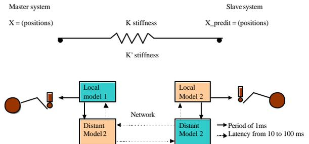
**Figure 5 Distant control of the robot in position**
