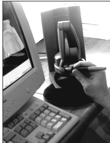
**Figure 1. The PHANToM haptic device in use**
