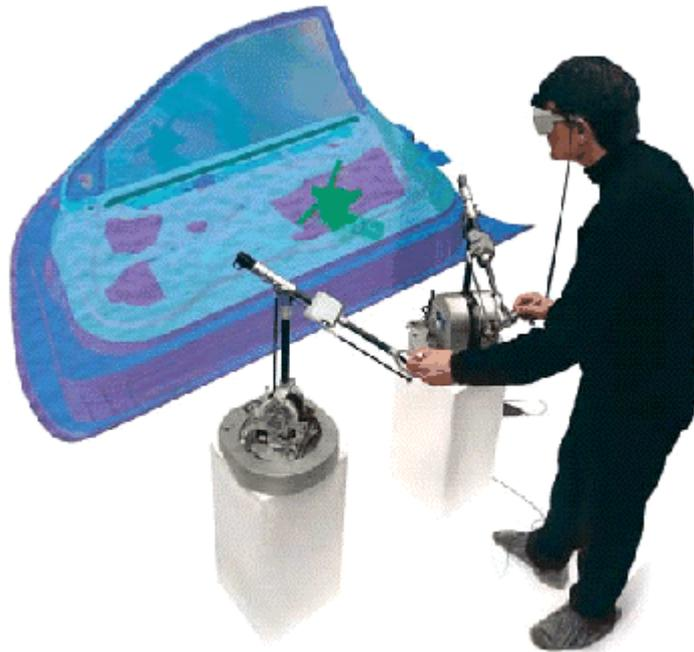
**Fig. 4.** The CEA PHARE virtual reality platform (rigid body prototyping instance): a stereoscopic workbench displays virtual environments, two haptic 6dof devices (VIRTUOSE 6D).
