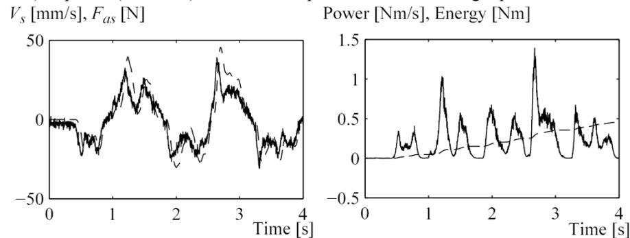
**Fig. 8.** Experimental results, slave in free space motion, force feedback turned off and low rate of change in the slave's control input  $F_{as}$ . The left plot shows the slave velocity  $V_s$  (dashed line) and slave input  $F_{as}$  (solid line), the right plot shows the energy (dashed line) and power (solid line) over the teleoperator controller's slave port
