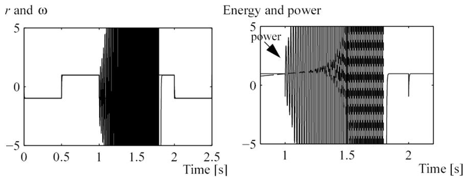
**Fig. 6.** Simulation results, left: Reference (solid line) overlapping the motor angular velocity (dashed line) and right: The energy (dashed line) and the power (solid line) of the system.
