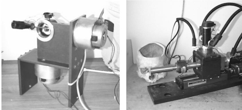
**Fig. 1.** System hardware, left: Master, right: Slave.
