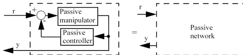
Fig. 4. Block diagram for illustrating the fundamental passivity result
