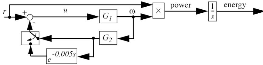
**Fig. 5.** System for the case study. Both systems  $G_1$  and  $G_2$  are passive and thereby also the feedback loop. Passivity is violated when the time delay is activated.
