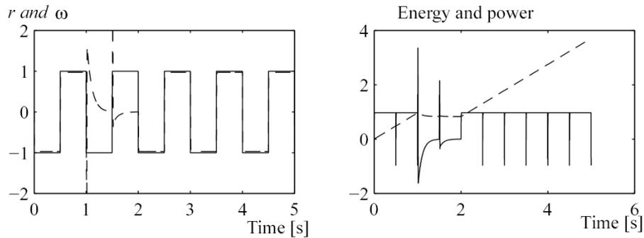
**Fig. 7.** Simulation results for the system in fig. 5 when the power controller is implemented. Left plot: The output (dashed line) and the reference (solid line). Right plot: The energy (dashed line) and the power (solid line).
