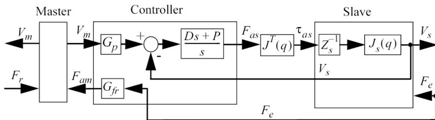
Fig. 3. The Force-Velocity teleoperator control structure.
