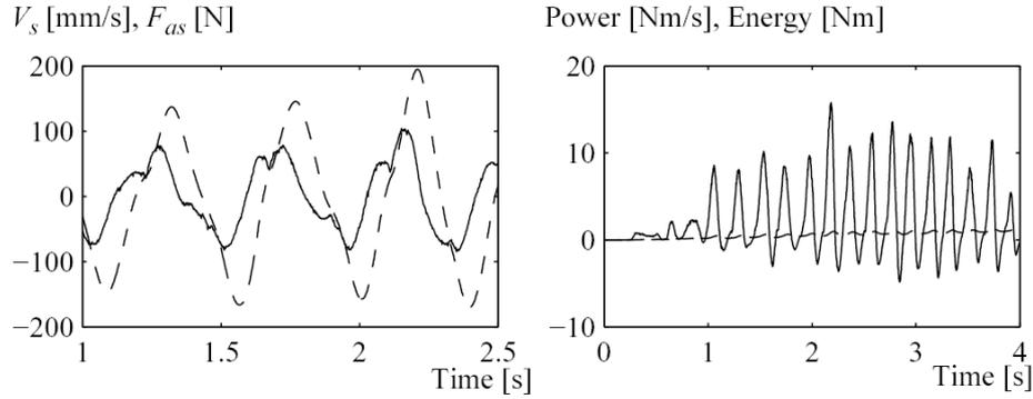
**Fig. 9.** Experimental results, slave in free space motion, force feedback turned off and high rate of change in the slave's control input  $F_{as}$ . The left plot shows the slave velocity  $V_s$  (dashed line) and slave input  $F_{as}$  (solid line), the right plot shows the energy (dashed line) and the power (solid line) over the teleoperator controller's slave port
