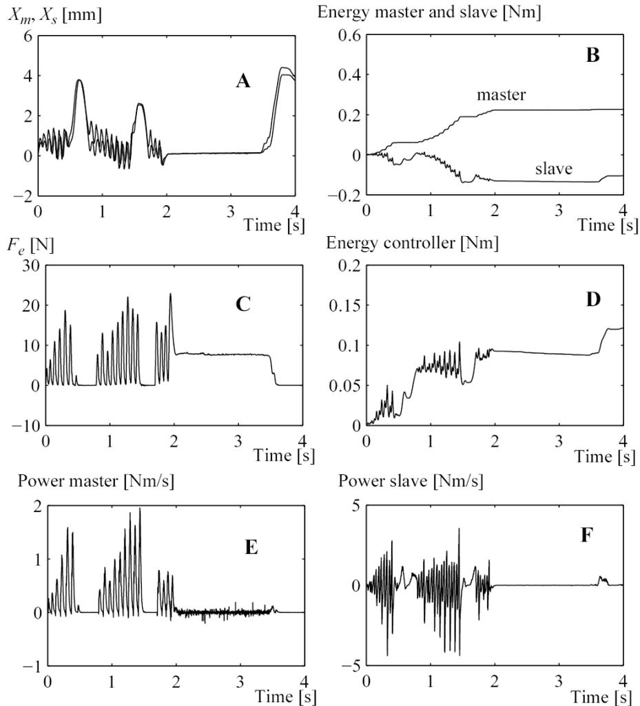
**Fig. 10.** Experimental results. Plot A: The positions of the master and slave. Plot B: The energies present on the controllers master and slave port. Plot C: The contact force. Plot D: The total energy on the controller. Plot E and F: The power on the controller's master and slave port respectively.
