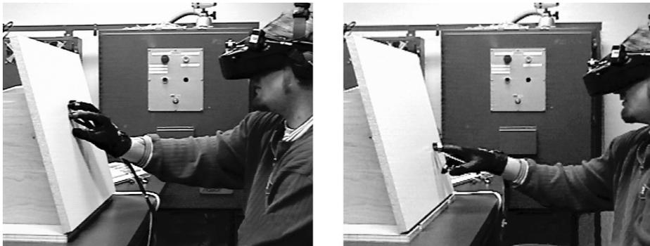
Fig. 2. External view showing the force-feedback glove and the static panel in the real world.
