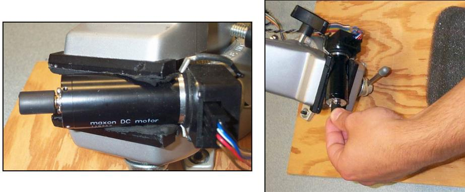
**Fig. 1. Haptic display and experiment setup.** A brass knob mounted directly on the motor shaft was covered with 1-mm rubber to prevent slipping while adding little compliance. The adjustable vise mount and cushioned armrest made the setup customizable and comfortable. Participants were asked to hold the knob lightly between thumb and index finger.
