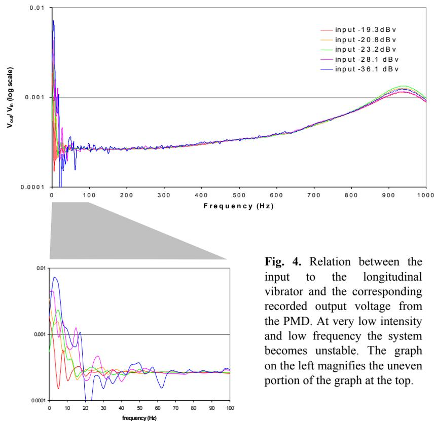
**Fig. 4.** Relation between the input to the longitudinal vibrator and the corresponding recorded output voltage from the PMD. At very low intensity and low frequency the system becomes unstable. The graph on the left magnifies the uneven portion of the graph at the top.
