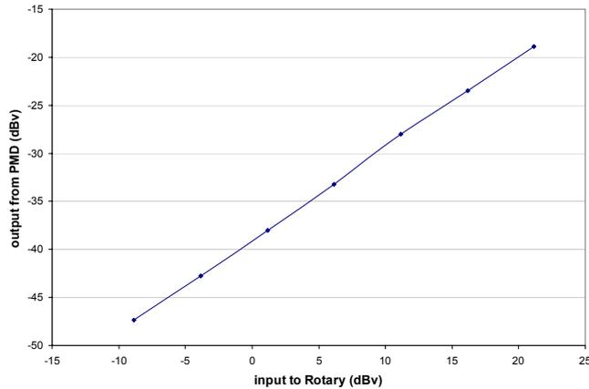
**Fig. 3.** Testing the linearity of the PMD where both input and output voltages are expressed in dB. Data collected from the rotary vibrator stimulated with 500Hz digitally generated sine-wave signal. The peak of the input voltage is equivalent to about 50dB SL rotary at 500Hz.
