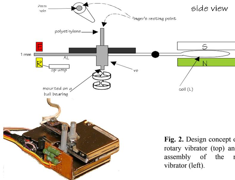
**Fig. 2.** Design concept of the rotary vibrator (top) and the assembly of the rotary vibrator (left).
