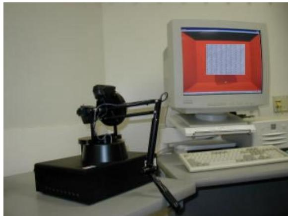
**Fig. 7.** PHANToM® haptic device.
