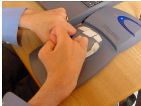
**Fig. 1.** The Logitech Wingman force feedback mouse.
