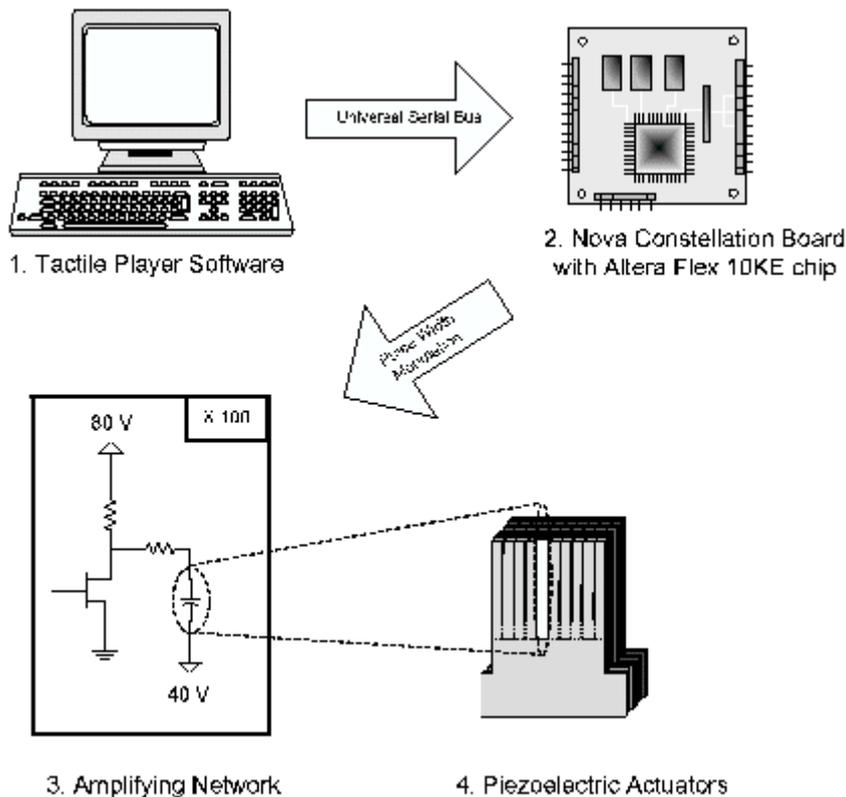
**Fig. 2.** The STReSS system is composed of four subsystems: A tactile player application (1) sends tactile images to the PLD (2). The PLD converts the tactile data into pulse width modulation (PWM) control signals used to drive a network of 100 switches (3). The switching amplifies control voltages to drive the piezoelectric actuators forming the tactile array.
