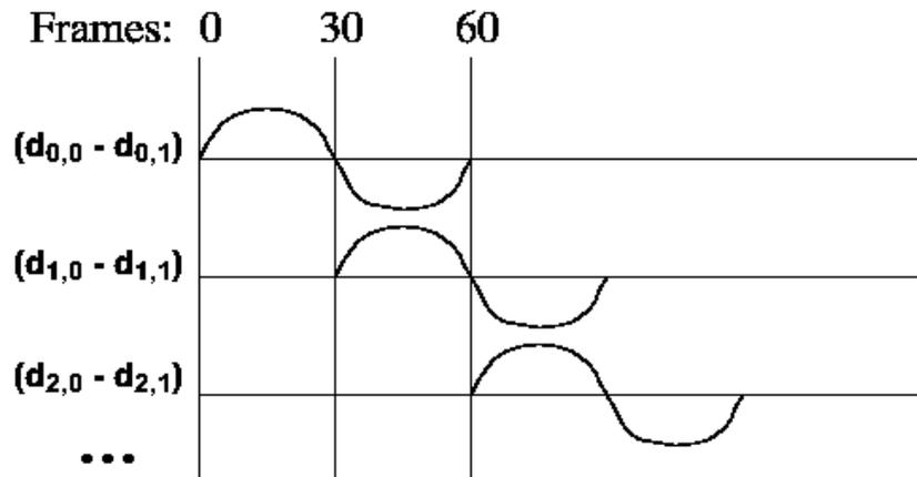
**Fig. 10.** Progressive wave activation for pairs of actuators, indicating the gap size variation through time and space.
