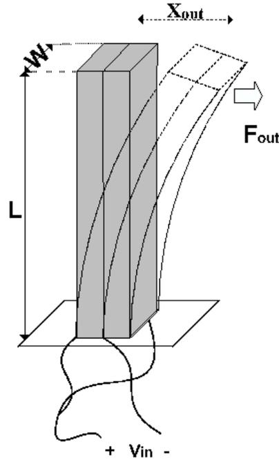
**Fig. 5.** Applying a differential voltage  $V_{in}$  between the middle electrode and the outside electrodes results in a lateral displacement  $X_{out}$  and a force  $F_{out}$  applied to the load at the tip of the bimorph. The bimorph has resonant frequency  $F_0$ . From basic cantilever mechanics, it is known that  $X_{out} \propto L^2$ ,  $F_{out} \propto W/L$  and  $F_0 \propto 1/L^2$ . Likewise, from basic electrical relationships,  $C_{piezo} \propto WXL$ .
