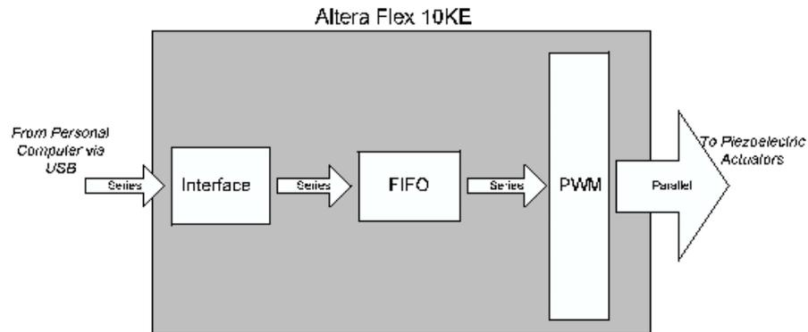
**Fig. 3.** The Flex 10KE is programmed to accomplish three functions: accept serial data from the USB interface, reconstruct images in a first in first out (FIFO) buffer, and generates 10 pulse width modulation (PWM) control signal.
