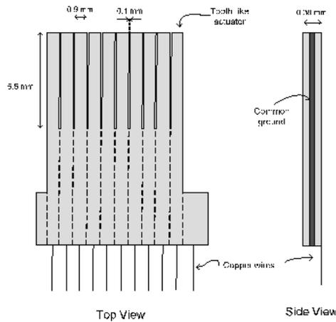
**Fig. 7.** Combe shape. Each tooth-like actuator is isolated from its neighbors by selectively removing the external electrodes. They all share the brass center shim as a common ground. Electric connections to the PCB are by small copper wires. Two shoulder are provided for clamping each combe in its socket slot. Sockets are made of two opposite racks attached to the PCM, as illustrated in figure 8.
