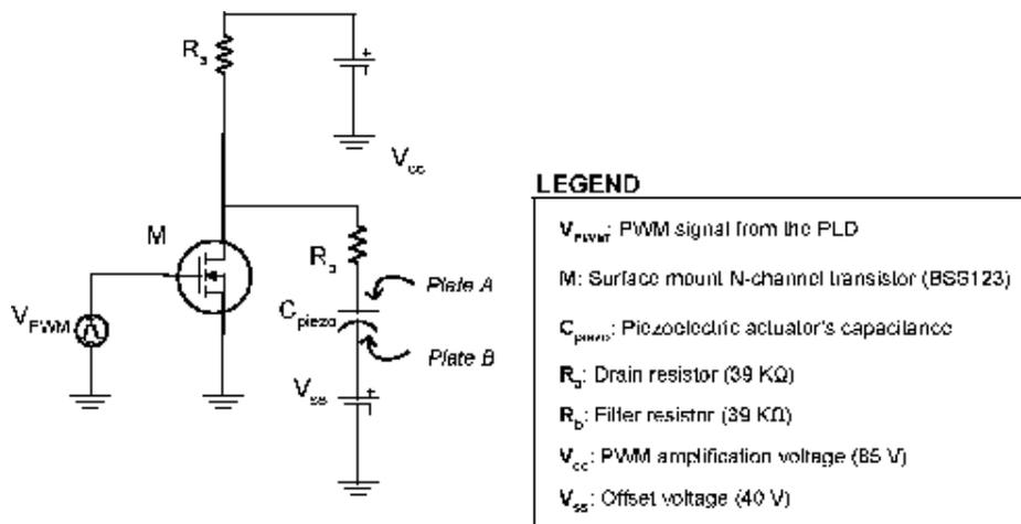
**Fig. 4.** An amplifying element comprises one transistor, two resistors and the piezo-electric actuator's capacitance. The 3.3 V PWMs are amplified to 80 V pulses before being filtered by the actuator. One of the piezoelectric's electrode (plate B) is offset by 40V so that bipolar potentials of  $\pm 40V$  can be sent across the actuator.
