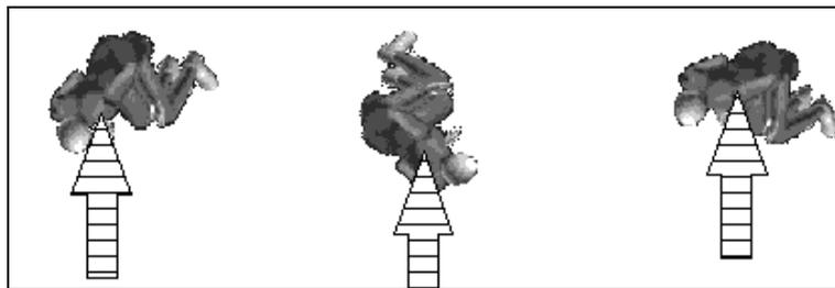
**Fig. 2.** Principle of projecting the artificial gravity vector as a localised vibration on the torso. A straight-up orientation will lead to no stimulation. For example, when oriented upside-down, the astronaut would receive a vibration on the shoulders. When the astronaut floats horizontally with his belly 'down', the vibration would be on the belly; and when floating on his back, the vibration would be on his back, etc.
