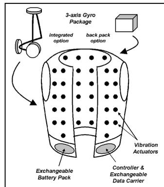
**Fig. 1.** Schematic lay-out of the multi-purpose vibro-tactile vest designed for use in the International Space Station (design by Dutch Space and TNO Human Factors, The Netherlands).
