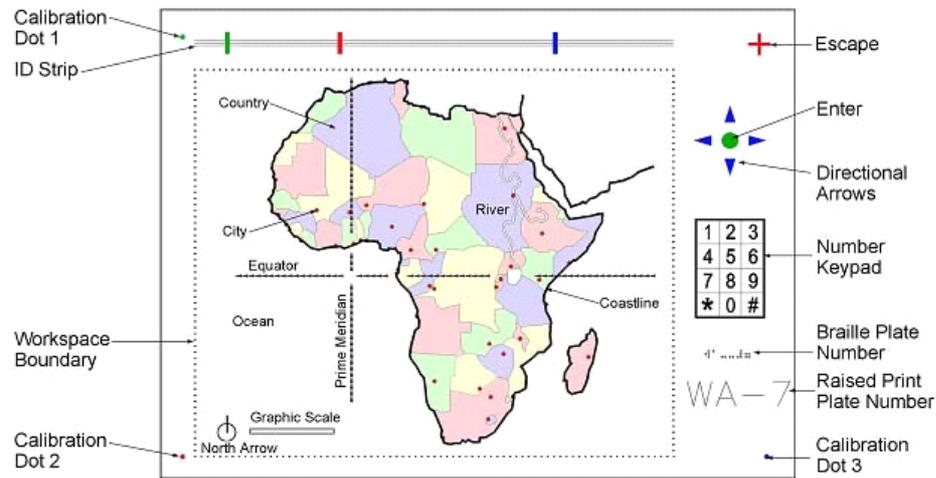
Fig. 2. Close-up of the tactile talking tablet
