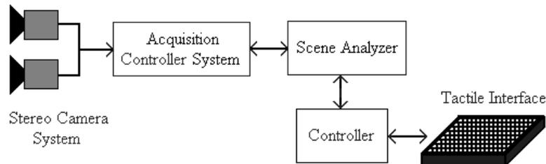
**Fig. 2.** IG-ETA system's global architecture.
