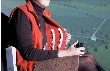
**Fig. 1.** Tactile Torso Display. The subject is showing the inside of the vest.
