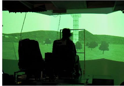
**Fig. 2.** View at part-task helicopter simulator showing NVG imagery.
