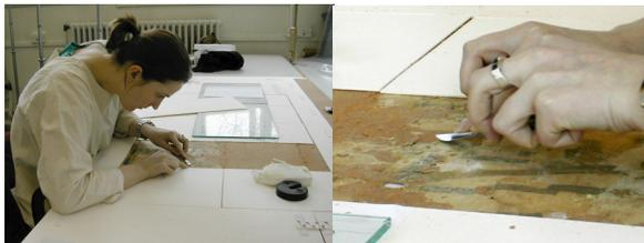
**Fig. 1.** A scalpel backing removal of hardboard from paper in progress
