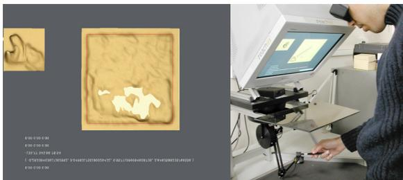
**Fig. 2.** The simulation prototype: a central square, deformable backing area (yellow) is positioned over a non-deformable paper layer (white). The layers share frictional characteristics. A smaller, but otherwise identical square, is provided on the left for the user to explore the simulation prior to commencing the main test area task.
