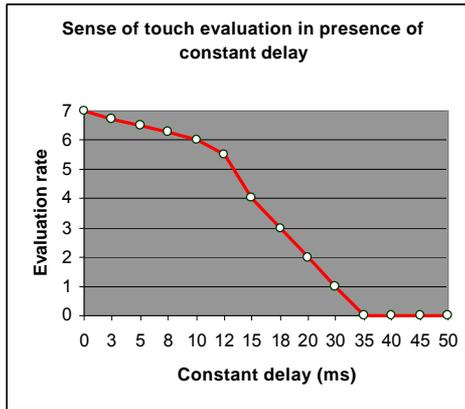
Fig. 3. Sense of touch evaluation in presence of constant network delay
