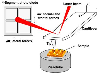
**Fig. 1.** AFM-force sensing: frontal and normal forces are measured in a coupled way.
