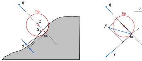
**Fig. 2.** Collision detection: Indentation depth and normal direction are obtained (left) and based on these, force directions can be derived (right).
