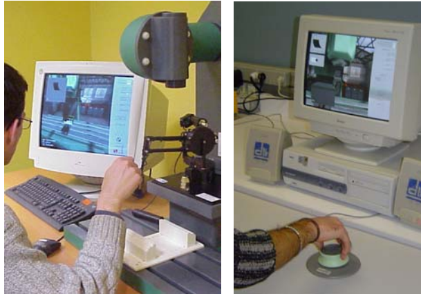
Fig. 2. (a) PHANToM-Based Solution (b) Pseudo-Haptic Solution with a SpaceMouse.
