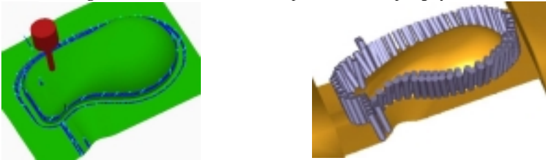
(a) computing pencil-cut tool orientations (b) tool orientation selection in a complex machining environment
