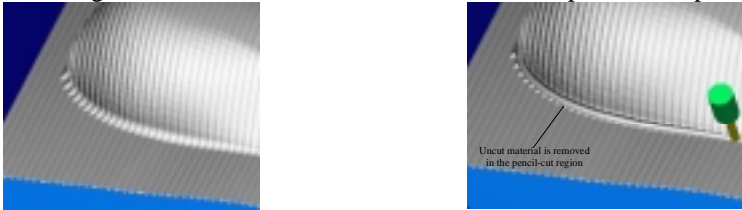
(a) Mouse model after finishing without pencil-cut (b) Mouse model during pencil-cut
