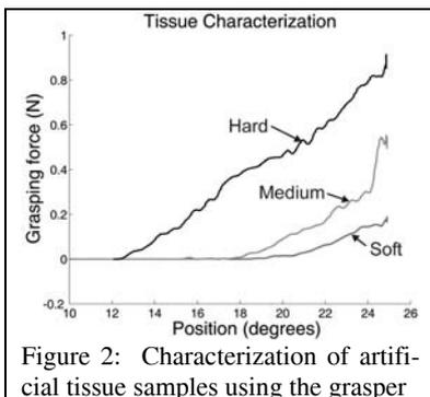
Figure 2: Characterization of artificial tissue samples using the grasper
