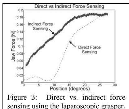
Figure 3: Direct vs. indirect force sensing using the laparoscopic grasper.
