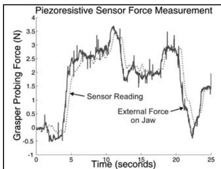
Figure 4: Longitudinal force measurement using the grasper compared to the actual forces during a probing task.
