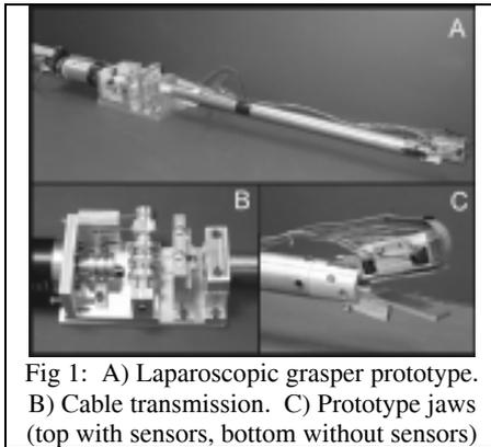
Fig 1: A) Laparoscopic grasper prototype. B) Cable transmission. C) Prototype jaws (top with sensors, bottom without sensors)
