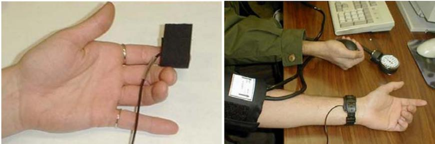
**Fig. 1.** A piezo pulse sensor is used for catching human pulse, attached on various position of human body, such as finger tip and wrist.
