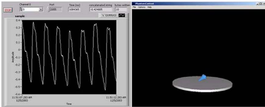
**Fig. 3.** Human pulse is captured, digitized and represented by replicated pulse (left). The haptically rendered leaping disk represents touch point where the pulsation is captured.
